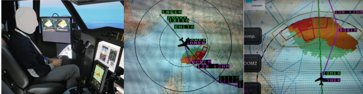
Figure 1: Position of EFB on the cockpit (right) (from [2]) and display of the classification results with identification of risk zones and route suggested to pilot. Two different display and zoom options can be used (center and right panels)
